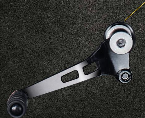
Precision shifts and quick launches come easy with the bottom mounted shift-lever and gears with negative back rack angle machined in all the gears lug to lug. Performance is taken up a notch by the quickshifter that saves milliseconds with every gearshift.
