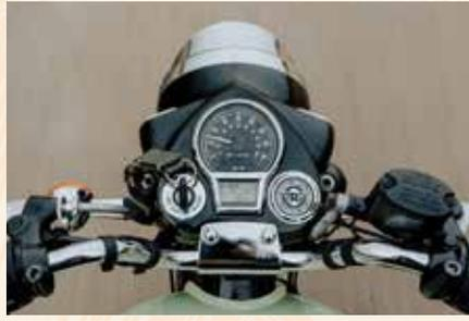
The instrument cluster combines the gracefulness of a 'dancing needle' analogue speedometer with the functionality of an LCD display.
