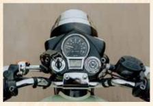
The instrument cluster combines the gracefulness of a 'dancing needle' analogue speedometer with the functionality of an LCD display.
