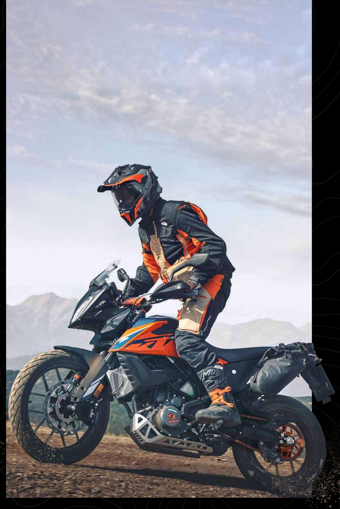
When the tarmac ends and the dirt track begins, KTM 390 ADVENTURE riders can simply switch to **OFFROAD MODE**. This allows a certain rear-wheel slip, meaning muddy puddles or thick sand is easily navigated.
