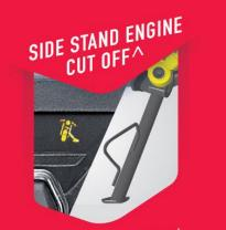
cuts off the engine when the side stand is engaged.
