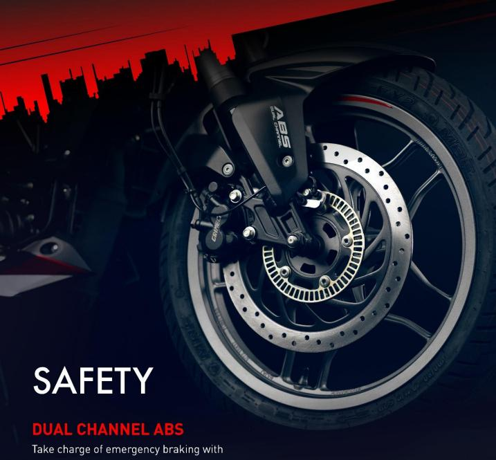
Take charge of emergency braking with absolute confidence. ABS comes into action ensuring wheels do not lock or subsequently skid on any surface.
